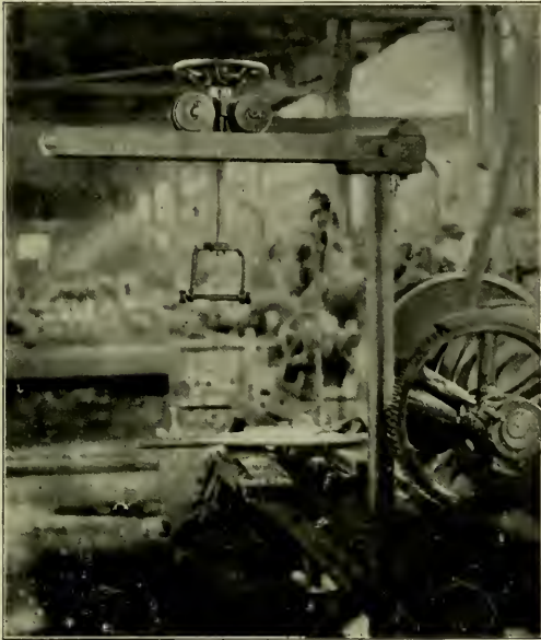
Fig. 17—Crane for Removing Heavy Lathe Chucks.
